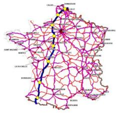
Figure 16 — 1020 km Calais-Bayonne 1 lane/direction + emergency lane (8 interchanges with the existing radial freeways) <sup>[33]</sup>
