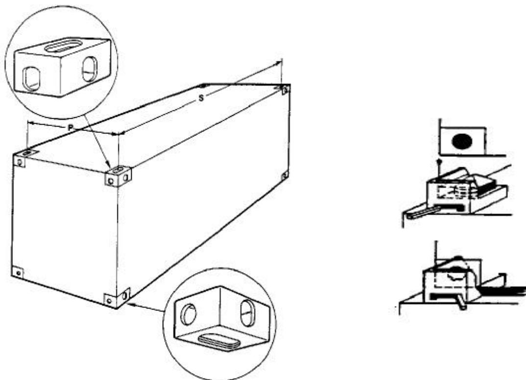
Figure 4: Corner fittings of the ISO container and the twistlock mechanism (sources: ISO/R 668 corner fittings, and SIS standardisation archive (1966), with kind permission from the NNI, Delft, and the SIS, Stockholm).
