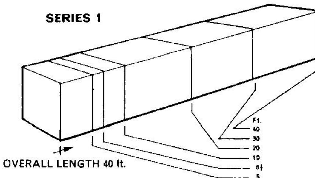
Figure 3: The first ISO Series 1 and Series 2 dimensions. (Source: Koster & Tilsley, 1968)
