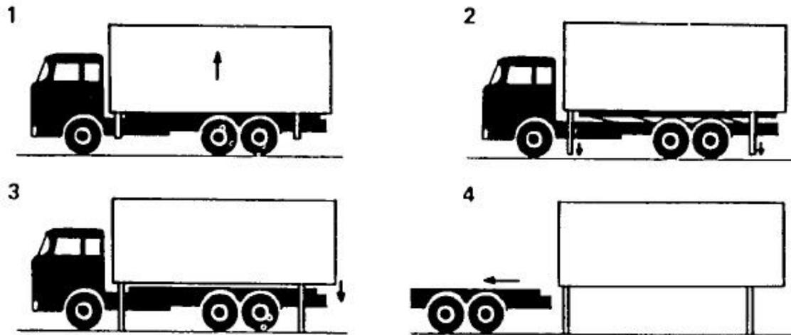
Figure 5: Unloading principle of the swap body. (source: Jensen, 1985, with kind permission)
