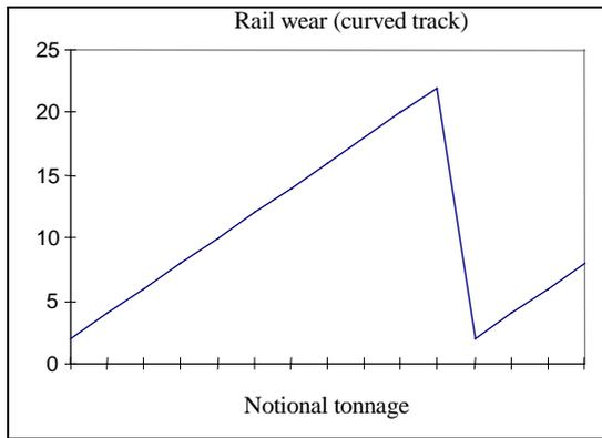
**Figure 3 Example change in quality (rail wear)**
