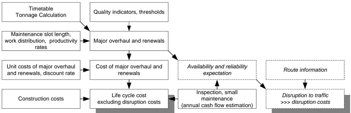
**Figure 5 Concept of the Life Cycle Cost Model**
