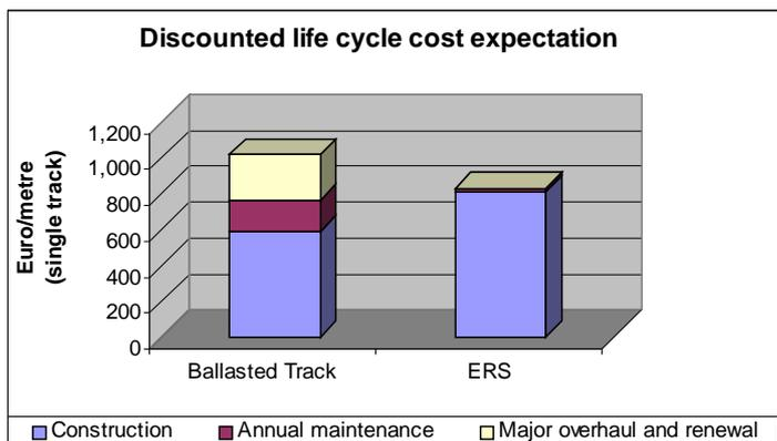
necessary *preparatory work* differ for different subgrades. Although construction costs of the railway track were about 40% higher than ballasted track, the total discounted life cycle costs were calculated to be 20% less than those of the ballasted track used in the Netherlands, which are about 2300 guilders per metre (figure 6). A rail renewal was not needed in the period considered and this means that only some annual maintenance is foreseen. Costs of inspection and
